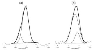
**Fig. 11.** Simulation diagram of O-1s XPS spectra of specimen **1**: (a) the  $1^{st}$  layer; and (b) the  $5^{th}$  layer.
