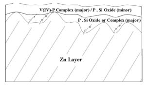
Fig. 16. Scheme of coating composition of specimen 1.
