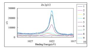
Fig. 14. Zn-2p XPS spectra of specimen 1.
