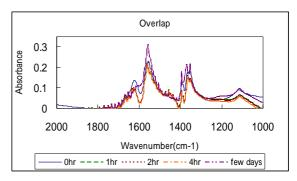
Fig. 8. FT-IR spectra of specimen 2 at various time intervals.
