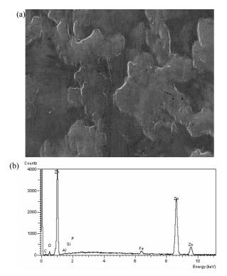
**Fig. 6.** (a) SEM morphology of specimen **1** with 0.5 mole aluminum ion; and (b) EDS results of the surface.
