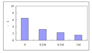
**Fig. 3.** Color difference ( L) of surface with various amount of aluminum ion.
