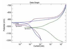
Fig. 1. Polarization curves of various specimens in the 3.5% NaCl<sub>(aq)</sub> solution.
