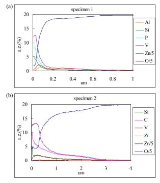
**Fig. 9.** GDS results of non-chromate coated GI sheets: (a) specimen 1; and (b) specimen 2.
