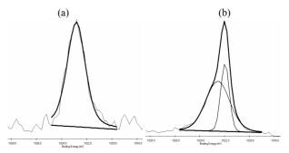
**Fig. 15.** Simulation diagram of Zn-2p XPS spectra of specimen 1: (a) the  $2^{nd}$  layer; and (b) the  $5^{th}$  layer.
