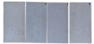
**Fig. 2.** Results of specimen **1** with various amounts of aluminum ion after black tarnish test; from left to right: 0.2, 0.5, 1, and 0 mole aluminum ion.
